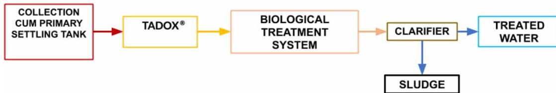
**Figure 1** | Schematic showing TADOX<sup>®</sup> Implementation at Pre-Biological Stage.
